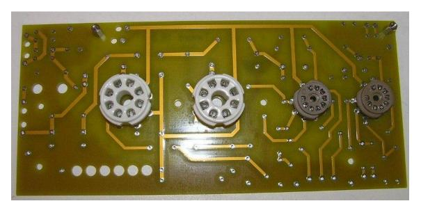
The tube sockets are installed as shown. The noval sockets only go in one way (on the back side). However, the octal sockets need to be properly oriented with the circuit board. Position the notch in these sockets so that they are pointing toward the two noval sockets.
