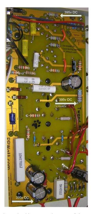
The unloaded B+ voltage should measure the same all the way up the power rail. A slight fluctuation is normal. If a difference greater than 5-10 Vdc is measured, something is drawing current when it shouldn't. Turn off the amp and troubleshoot the problem.
