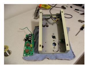
Salvage the ground wire from the stock circuit board for use later.
