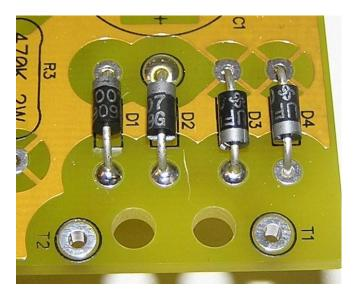
If you are using a center-tapped PT, like the MPS 325.2, Weber 025130 or Edcor XPWR107 you only use the 'first' two diodes, D1 & D2. (If you use all 4, you'll put way over the top voltages into the circuit... Don't do it!)
