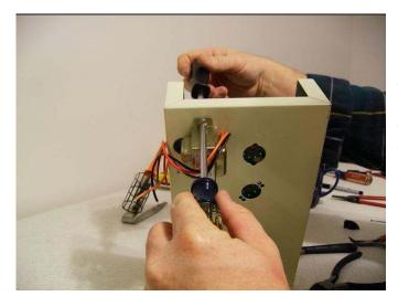
Keep the output jack board with it's ground wire attached.
