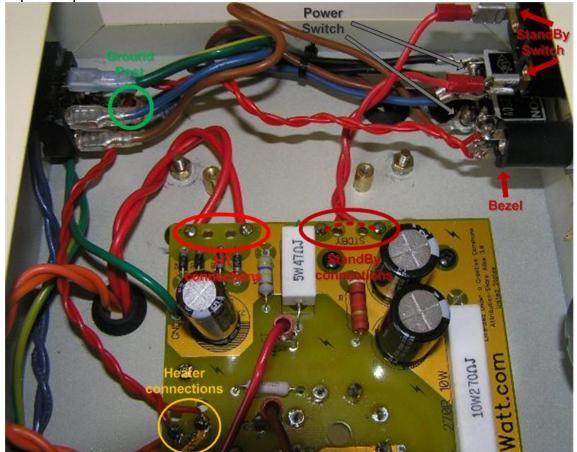
The orange wires from the PT go to the heater pads. I route them from underneath & up, soldering from the top side of the PCB. The thin wires you can see soldered to these same pads go to the 6v Bezel. If you have a 120/240v lamp you'd take some taps from the power switch.
