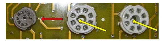
Tape the sockets (with sticky tape) 'flat' to the chassis. You are going to invert the chassis back up to solder them on to the PCB, so if you don't the tube sockets will fall back out again!
