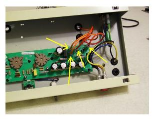
Remove the six (6) screws fastening the circuit board to the chassis. Keep them. You'll use them to attach the new PCB.
