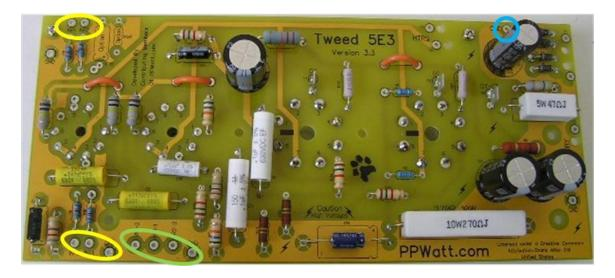
The input jack wires connect to the pads marked in yellow.
