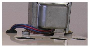
hole & the input wires go through the new hole as shown. I use a couple of washers with the bolts to raise the OT up from the chassis a little. I find it sits better this way with the wires not squashed up against the chassis.
