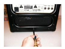
Locate the screw caps on the top of the EVJ. Using a standard screw driver, the smaller the better, pry up the caps until you can pull them out of their sockets.
