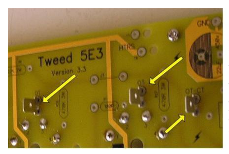
Extra solder time is necessary to heat the spade connector before solder will flow. Hold the iron on the connector. Feed the solder when the joint is hot enough to flow. Straighten the connectors as the solder joint sets, or hardens.
