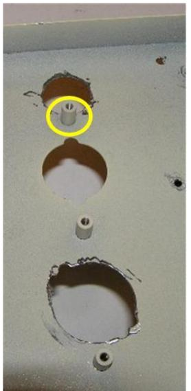
You want to drill the Noval (9-pin) holes so that the socket 'lip' rests against the chassis. The Octal (8-pin) socket holes need to allow the socket to slip all the way through.
