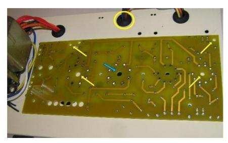
Mark the existing stand-offs so that you can use them to line up the PCB & then lightly tape it to the chassis.
