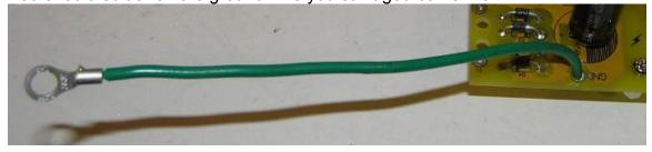
This will be connected to the existing ground post. You will note that the mains ground wire from the IEC connector also connects to this post. Some people say it is better practice to have a separate ground for that wire than the star ground for all the others.
