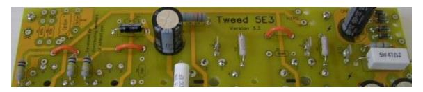
Finally, the last of the resistors! Note that R7 & R8 are not installed on the PCB. They are part of the input jack complex.
